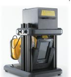
print and email from the X-50 and connect to virtually any information system for real-time data. On-board macro camera allows for photo-documentation of materials tested, and the Bluetooth label printer provides instant hard copy labels.
