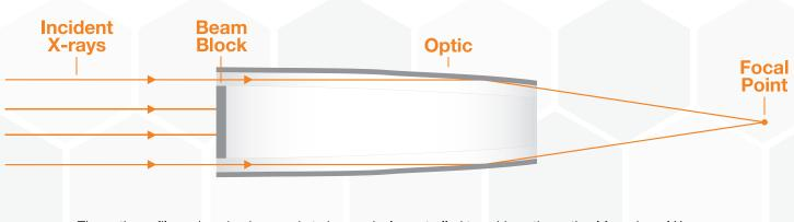
The optic profile and packaging needs to be precisely controlled to achieve the optimal focusing of X-rays.
